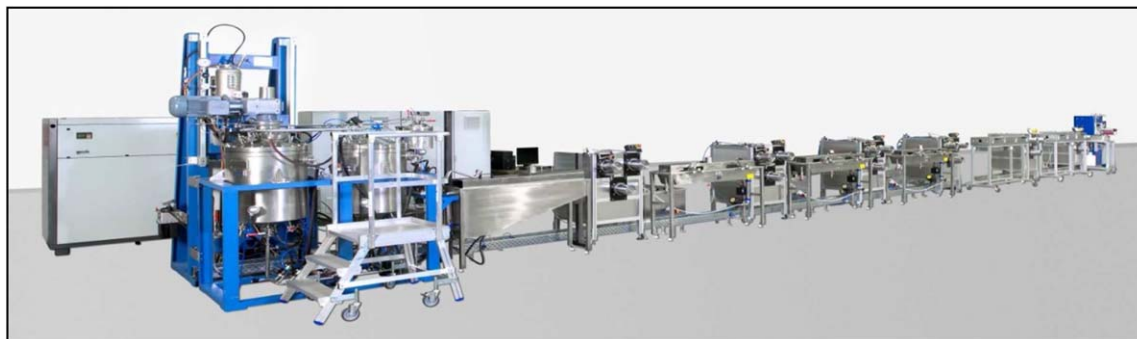
Figure 3. Wet-spinning pilot plant by Co. Fourné Polymertechnik GmbH, Germany. [Color figure can be viewed in the online issue, which is available at wileyonlinelibrary.com .]
